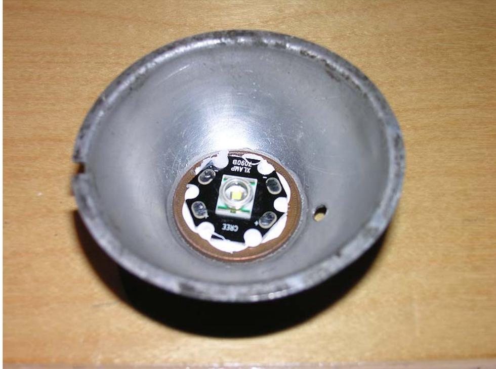
The next stage was to install the Q5 emitter with lots of thermal paste. I also drilled a small hold in the side of the reflector to allow the wires to pass through from the rear to the Q5.
