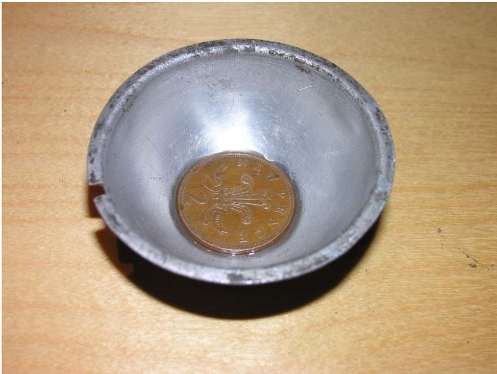
With the metal reflector out, I needed a firm base on which to mount the Q5. This would have to be flat and able to let heat move out and away as efficiently as possible. I opted to glue down a 2p coin, as it's round, copper (good heat conductivity) and just the right size. I used superglue just to hold it in place then plastered it in thermal paste to allow heat to pass from the coin to the reflector smoothly. Not a small heatsink by any means!
