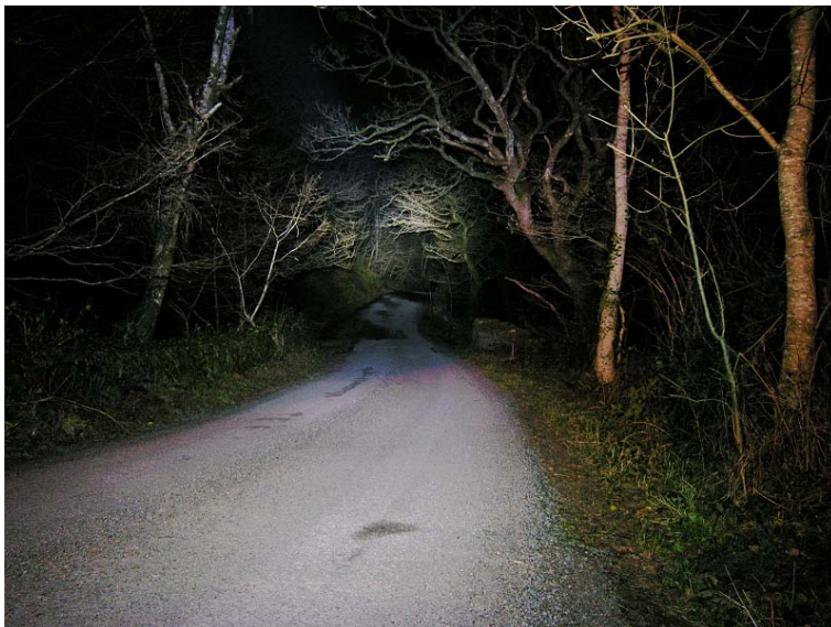
Homemade Q5 Caplamp: "Holy Boat Anchors, Batman!" The centre spot is much brighter, travelling far further. The spill is also far wider meaning it's going to be nicer to walk with. Absolutely stunning output.
