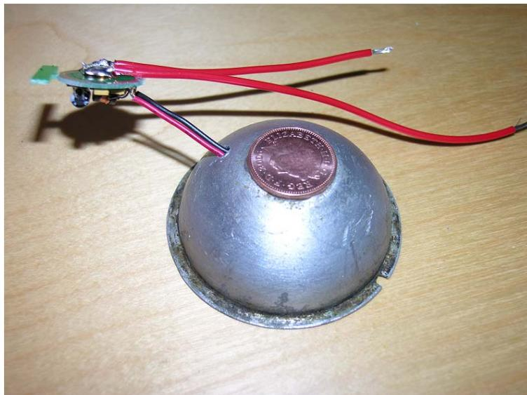
I was worried the wiring would come apart on the regulator when I pushed it all into the head, and also worried it could short out. So I wrapped it in heat-shrink and put a cable-tie around it to give it more strength. I also put insulated crimp-terminals on the wires connecting it to the head so it could be removed easily at a later date.
