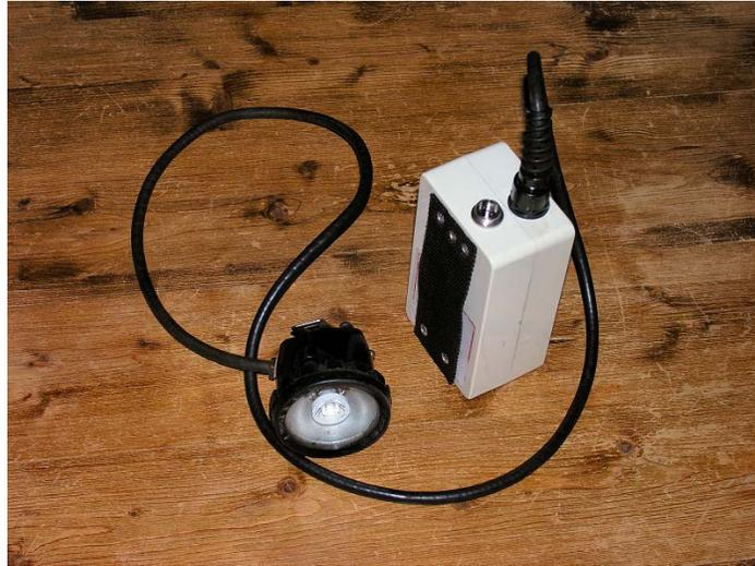
At the time of writing, the newly released Cree Q5 LED is the brightest LED ever made. When consuming about 3.7 watts of power, it produces around 230 lumens of light. Compare this to the traditional halogen Oldham caplamp bulb, which consumes 4 watts of power and produces only 48 lumens of light. A rather uneven yellow light at that. Even the now positively outdated Luxeon III LED yields only 90 Lumens from 3 watts of power consumption - so the new Q5 really is streets ahead.
