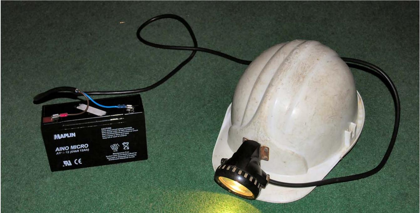
The weak point in this setup as any hardened mine-explorer will immediately notice, is the cable joining the battery. Normally on a Caplamp, the battery has loops so that it can be safely hung from a belt, and the cable is held very securely to prevent it from being pulled off the battery in the event of a snag.
