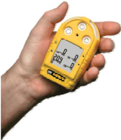
Gas detectors come in all shapes and sizes from single gas to multi gas. But as a mine explorer you will need at least a 4 gas type for it to be any good and give you a good level of protection.
